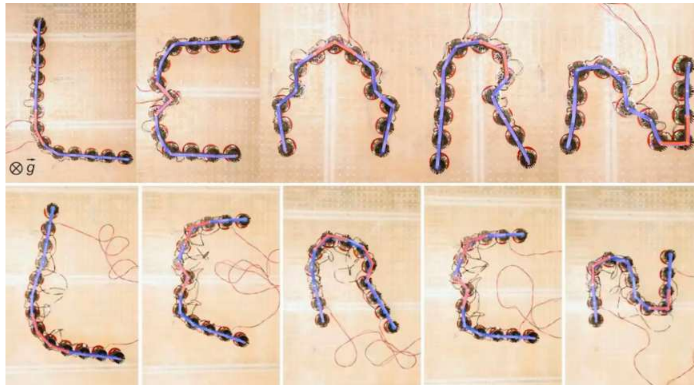
Top, A robotic metamaterial spells the word 'LEARN'. A metamaterial is a special material whose properties are not determined by its chemical composition alone but also by its structure, giving rise to unusual properties. COULAIS LAB/UNIVERSITY OF AMSTERDAM
